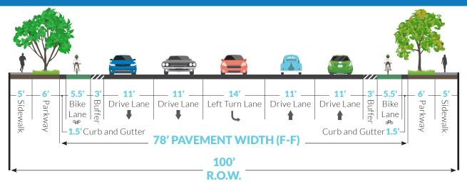
\*Minor arterials can also include a raised median in place of a center turn lane.
