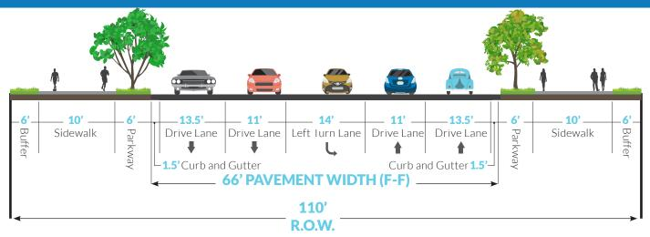
\*Principal arterials can also include a raised median in place of a center turn lane.
