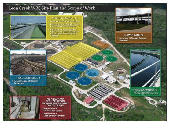
Rehabilitation of the San Antonio **Water System Leon Creek Water Recycling Center** involved multiple components, including automation of the aeration system and chlorination/ dechlorination system, plus repairs to the clarifiers and construction of a blower enclosure.
